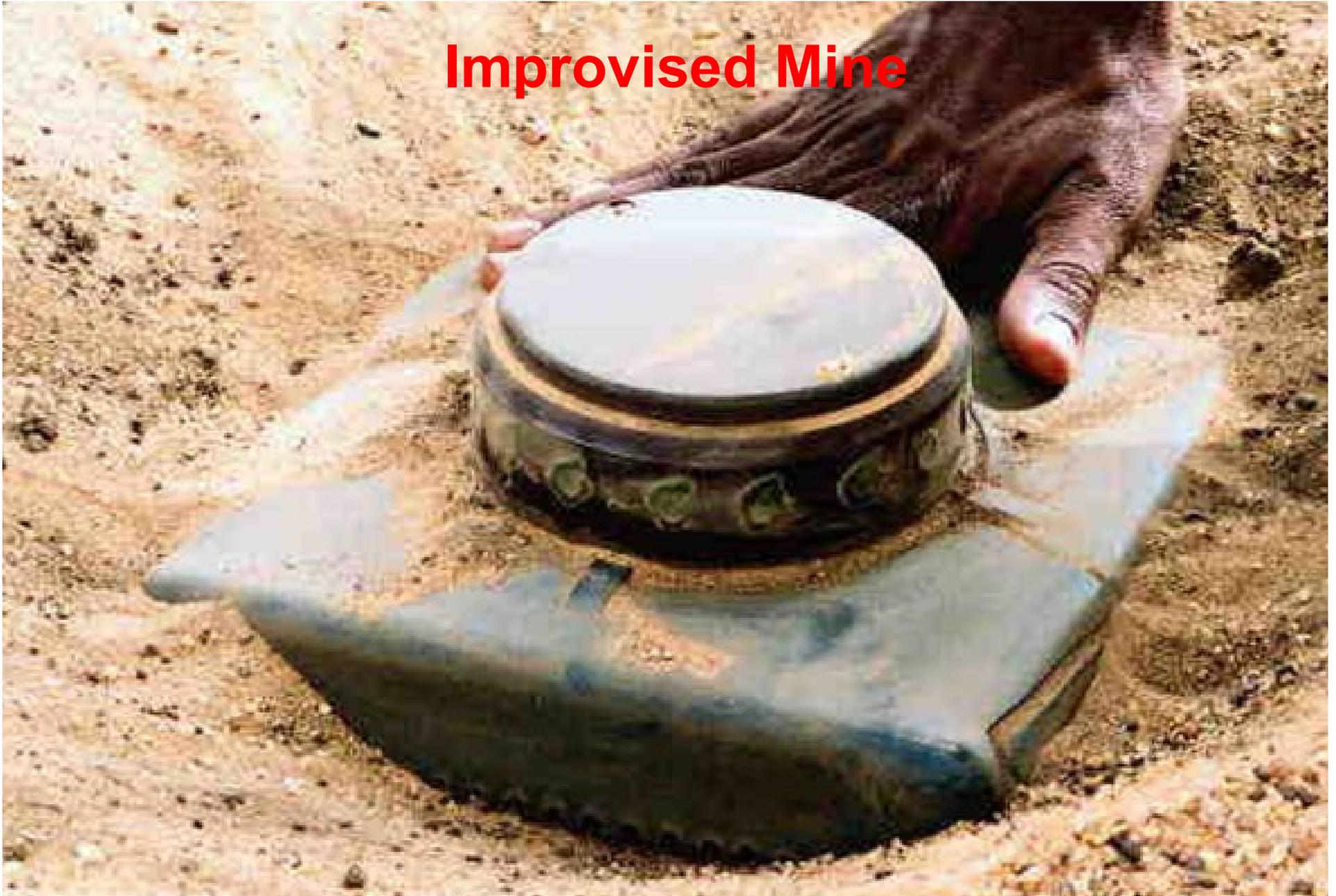
In Mali, operators have found anti-tank mines with some shear pins drilled out, so that lighter-weight civilian vehicles will initiate it.
